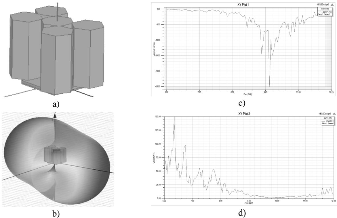
Fig. 2. The first version of the quasifractal DRA: a) – power scheme; b) – BP; c) – AFC; d) – VSWR
