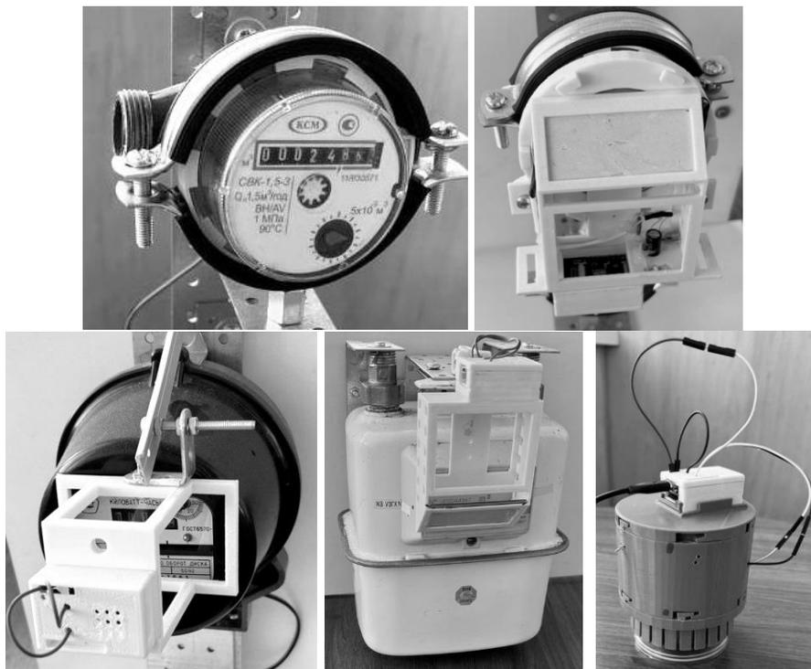
Figure 14: Options for mounting it on meters
