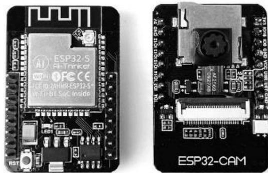
Figure 13: ESP32-CAM
