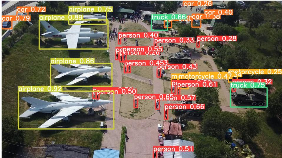
Fig. 6. Object detection in an aerial photograph from the VisDrone set in Colab Notebooks using the YOLOv5x model
