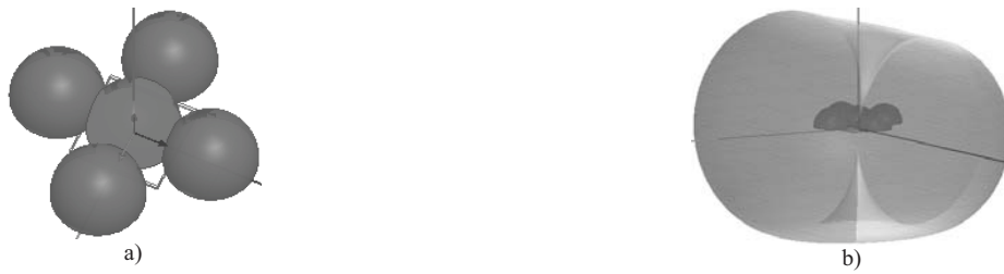
Fig. 5. Quasi-fractal hemispherical DRA with overlapping constituent elements in 10 mm: a) – layout; b) – BP
