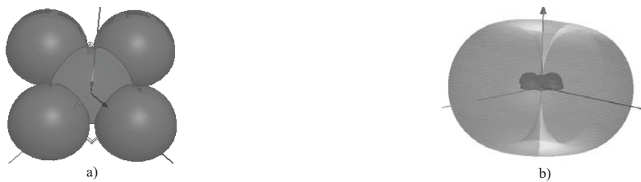
Fig. 7. Quasi-fractal hemispherical DRA with overlapping constituent elements in 20 mm: a) – layout; b) – BP
